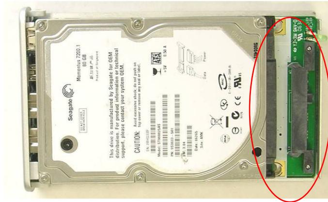
5. You may need to angle the drive as you push it into place. After connecting the drive to the SATA interface on the circuit board, the drive should lay flat on the board.
