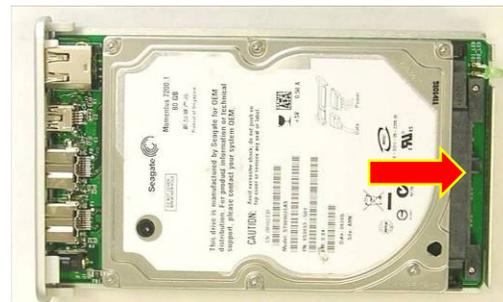
6. Secure the drive in place using the included screws. Drive the screws through the bottom of the circuit board and into the hard drive.
