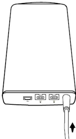
Connect the USB or FireWire cable to the corresponding port on the ToughTech mini.
