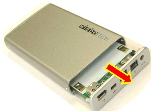
3. One drive screw is already inserted into the circuit board to prevent movement during shipment. You'll need to remove this screw before you can install the hard drive. The screw is held in place by a plastic nut.
