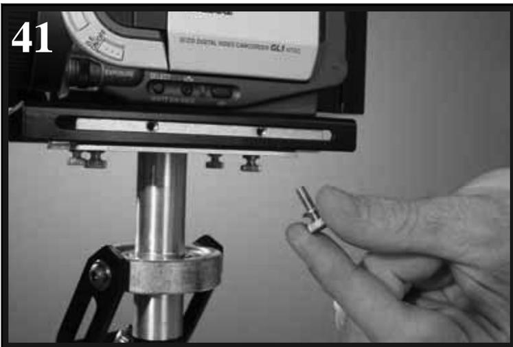
Insert and secure the four remaining BRASS THUMB SCREWS through the slots in the HEAD PLATE and into the “Threaded Inserts” in the sides of the MID PLATE.
