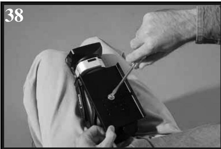
With your Camera base side up in your lap and with the HEAD PLATE in place, use a flat head screwdriver to secure the HEAD PLATE to your Camera using the CAMERA MOUNTING SCREW and ¼” WASHER combo you have just selected.
