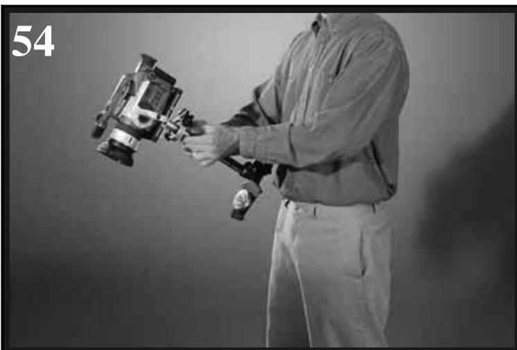
You can also attach an external LCD Monitor to the accessory shoe on top of your Camcorder. We believe that better results are obtained when you attach the Monitor to the 2000 Pro’s base, because this way you generally have to look slightly down to see the Monitor, and in doing so your feet are more visible to your peripheral vision. This makes negotiating obstacles with the 2000 Pro safer.
