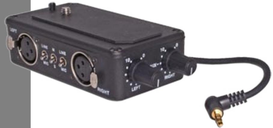
*The BeachTek DXA-4 is a two channel, transformer balanced XLR adapter for the Sony VX2100 and FX1 camcorders. The DXA-4P is identical in features but designed for a perfect fit on the Canon GL1 or GL2. These adapters are designed to easily attach balanced or unbalanced type microphones to your camcorder. The DXA-4 and DXA-4P gives you all the benefits of using balanced audio devices for clean audio as well as control over the signal levels to ensure the best possible sound recording.*
